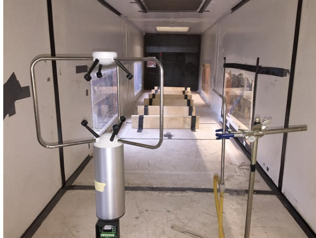
Figure 2.17: The view of R.M. YOUNG 81000 (left) and Pitot tube (right) at wind tunnel.
