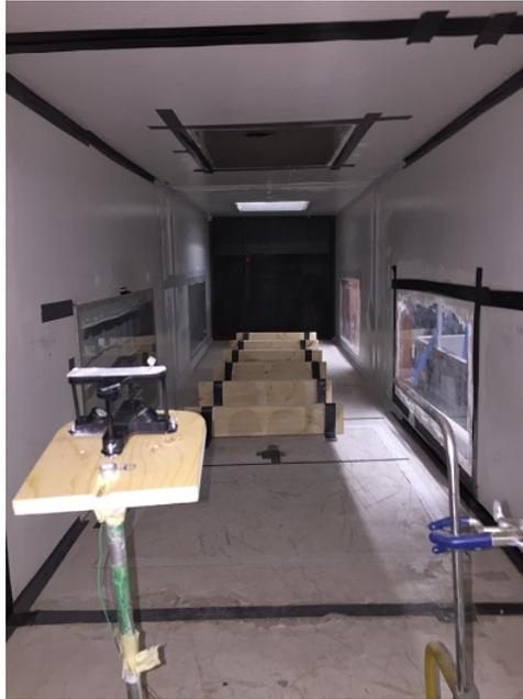
Figure 2.15: The view of TriSonica™ Mini (left) and the Pitot tube (right) in wind tunnel.
