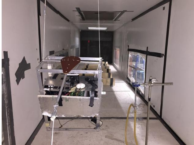
Figure 2.18: The view of gondola and Pitot tube at the wind tunnel.
