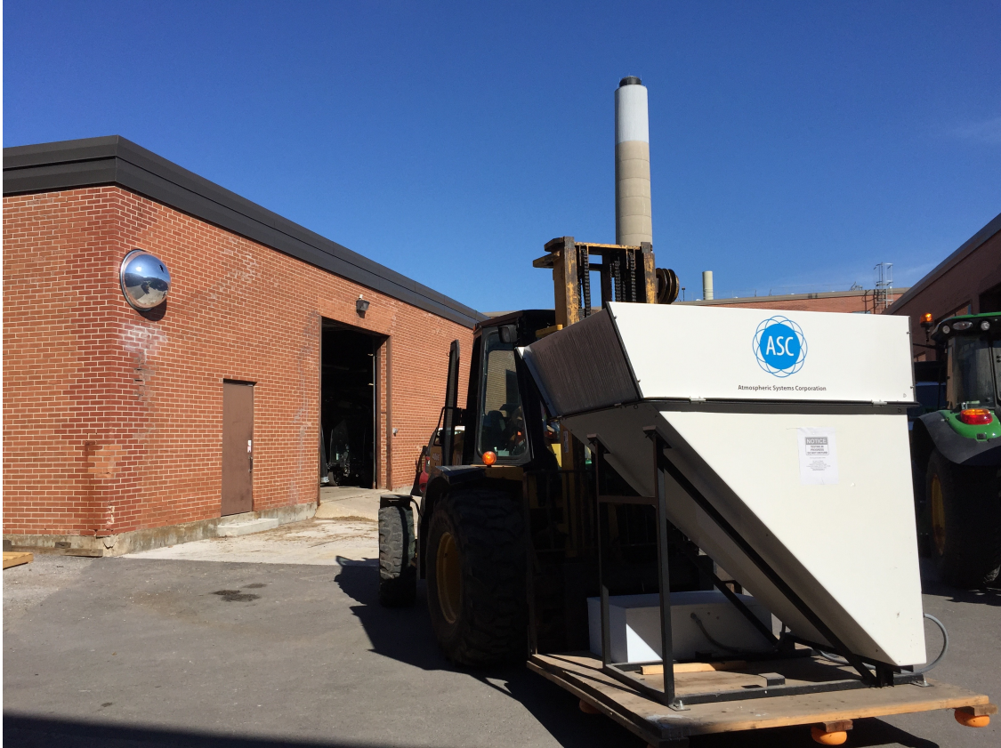
Figure 2.3: mini SODAR used at the site; photo courtesy of Dr. Amir A. Aliabadi.
