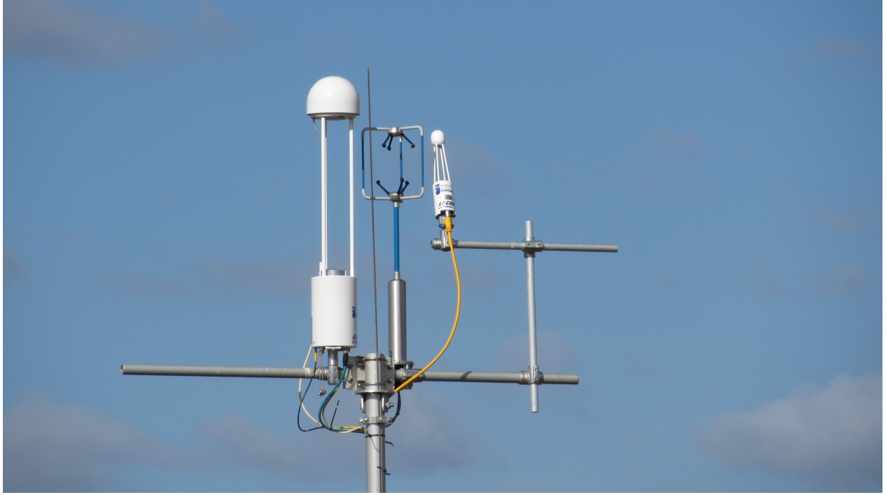
Figure 1.2: An eddy covariance sensor used to measure GHG emissions from an open-pit mining facility; photo courtesy of Dr. Thomas Flesch.
