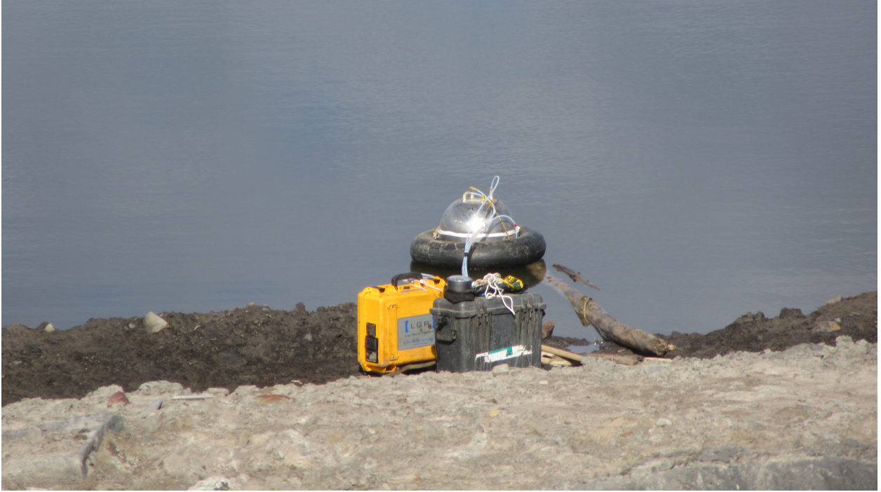
Figure 1.1: A flux chamber used to measure GHG emissions from a tailings pond in an open-pit mining facility; photo courtesy of Dr. Thomas Flesch.
