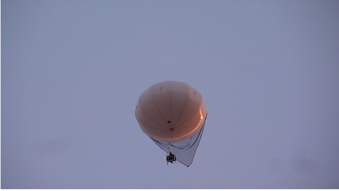
Figure 2.4: Tethered And Navigated Air Blimp (TANAB) used at the site; photo courtesy of Dr. Amir A. Aliabadi.
