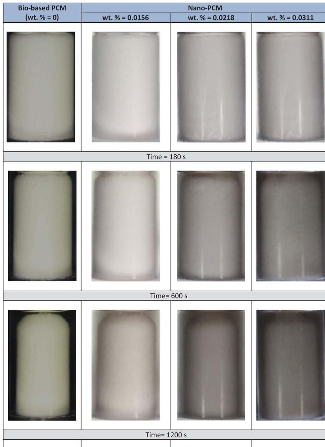
Fig. 2. Visualization comparison of bio-based PCM (wt.% = 0) and different nanoparticles weight fractions (wt.% = 0.0156, 0.0218, and 0.0311), H = 7.2 cm.
