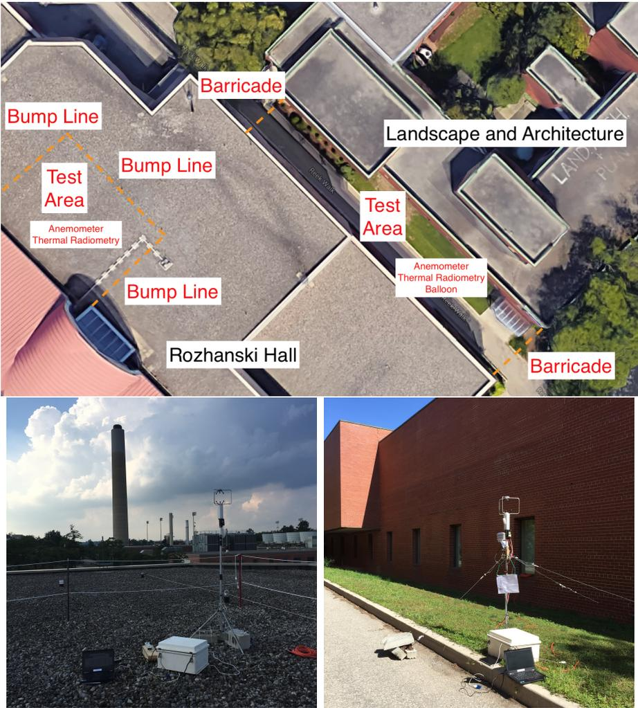
Figure 1: University of Guelph micro-climate campaign in August 2017: campaign site (top); station 1: sonic anemometer installation on the roof of Rozhanski Hall (bottom left); station 2: sonic anemometer installation on the street of Reek Walk (bottom right).
