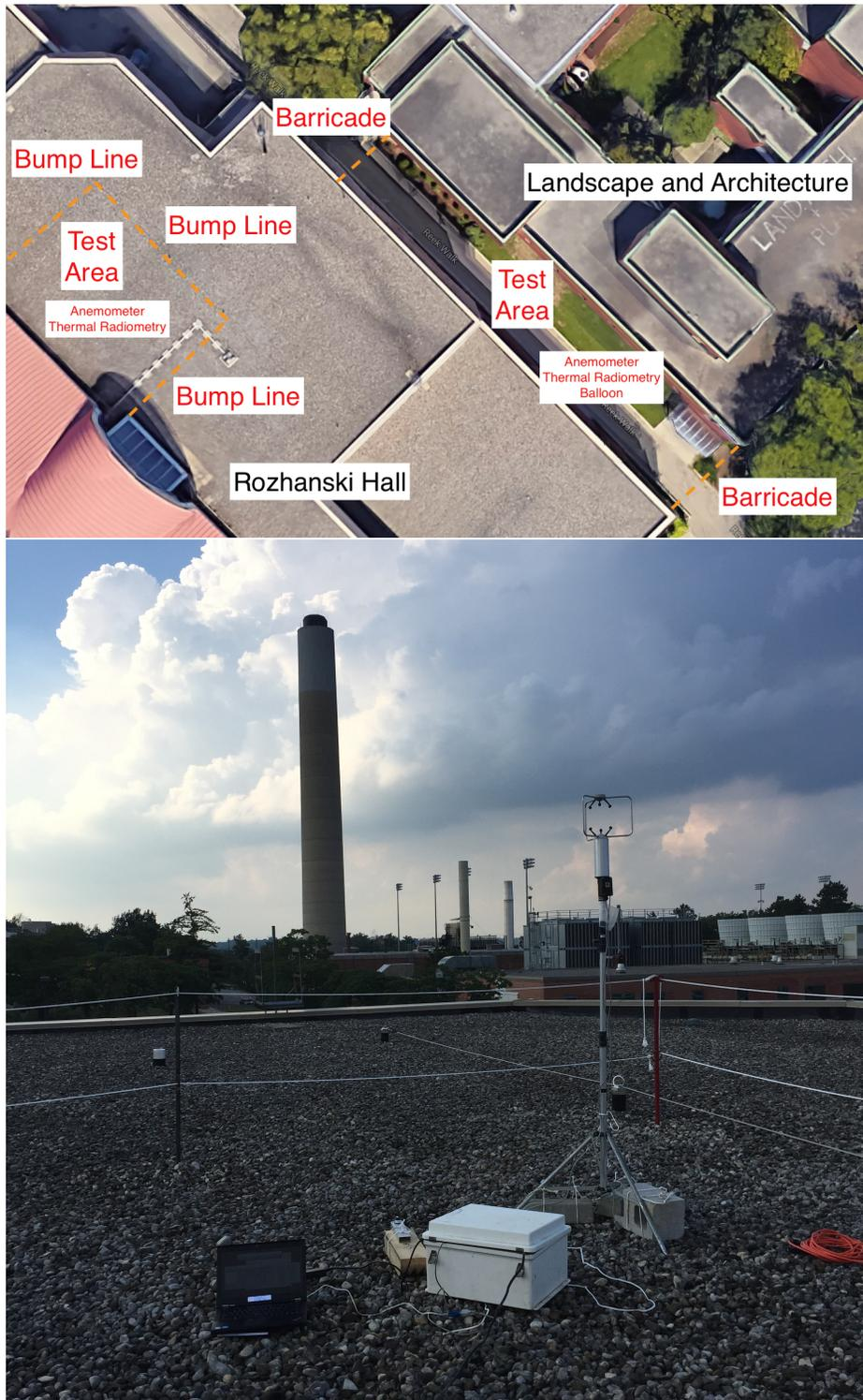
Figure 1: University of Guelph micro-climate campaign in August 2017: campaign site (top) and sonic anemometer installation on the roof of Rozhanski Hall (bottom)
