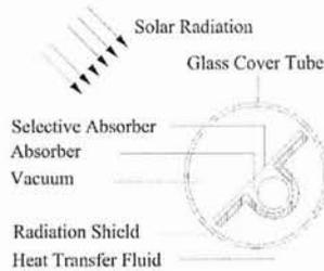
Fig. 2. Solar collector schematic
