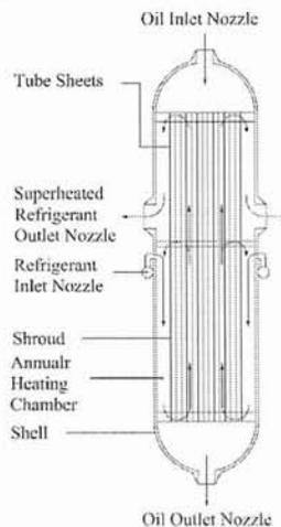
Fig. 4. Boiler schematic [2]
