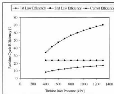
Fig. 5. R123 ideal Rankine cycle efficiency, 2<sup>nd</sup> law efficiency, and corresponding Carnot cycle efficiency
