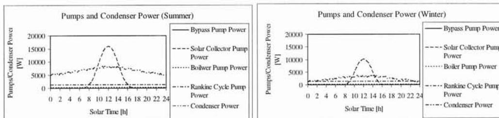
Fig. 11. Parasitic losses for pumps and fans
