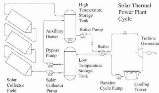
Fig. 1. Solar thermal power plant cycle
