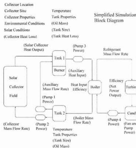
Fig. 7. Simplified simulation block diagram
