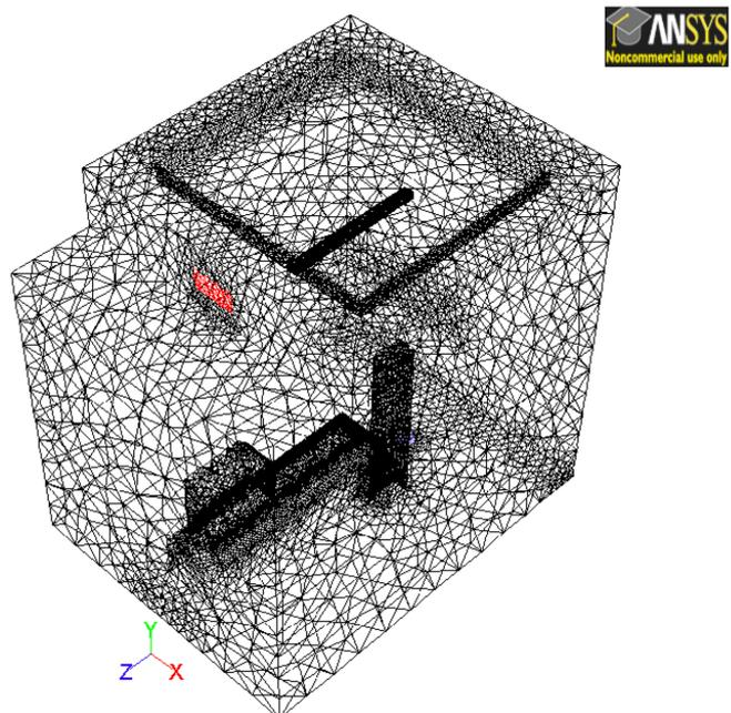
**Figure 2.** Numerical mesh for case 1
