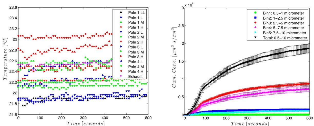
Figure 3. Temperature stratification (left) and exposure at breathing zone (right) for case 1
