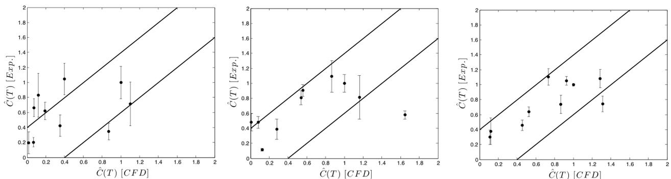
**Figure 4.** Measured [Exp.] and predicted [CFD] normalized exposure at sitting (left), breathing (mid), and upper (right) zones for short time ( $T=140$  s)
