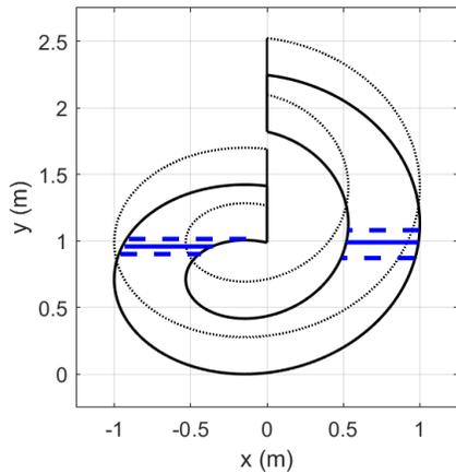
Figure 10. Visualization of water level within one bucket during transit of bucket from inlet to outlet. ( $D_o = 2$  m scale-screw with a surface roughness of  $n = 0.014$ .) Observing bucket in the  $x$ - $y$  plane in the  $+z$  direction (cf. Fig. 8). Solid blue lines are mean free-surface level, while dashed blue lines indicate the maximum and minimum levels observed.
