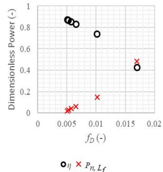
Figure 8. Dimensionless power as a function of surface roughness. Dimensionless power production is given as the mechanical efficiency ( $\eta$ ) and frictional loss ( $P_{n,Lf}$ ) is non-dimensionalised with a similar approach.
