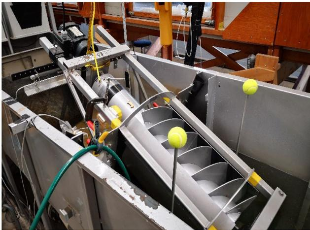
Figure 3. University of Guelph Archimedes screw apparatus.
