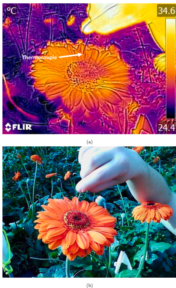
Fig. 4. (a) Thermal image analysis of a Prestige flower recorded on January 24, 2020, where temperature is displayed as degrees Celsius and the white arrow indicates the tip of the thermocouple; (b) corresponding digital image of the Prestige flower recorded by digital camera of the FLIR E6.
